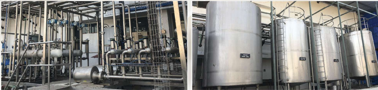
Four Circuit C.I.P. System
